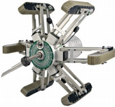
Cleaning Robot (basic setting for round ducts)
